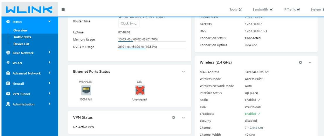
Figure 2-2 Router Status GUI
